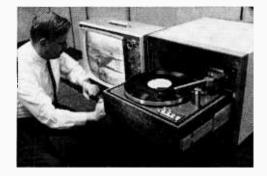
One picture is read out repeatedly and displayed during the time that the next one is being formed from the video information in the grooves of the recording.
