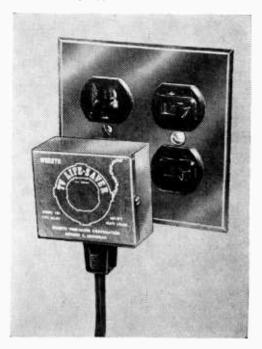
and the TV set plug is inserted into the gadget. When the set is first turned on, a resistor is connected in series with the AC line to cut the voltage reaching the set. After the resistor gets hot, a pair of contacts close and full voltage is applied to the set. It should greatly increase tube life.
